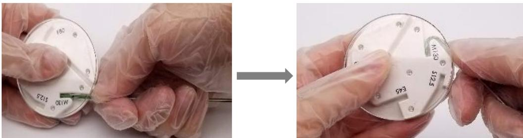
14. Inspect the device to ensure no damage incurred and the desired bend angle was achieved.
